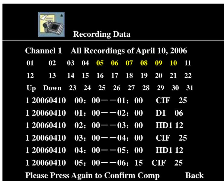
Press **【CF】** key again, if the capacity of CF card is smaller than the capacity of the period of time, “Ineffective” will display; If the capacity of CF card is not smaller than the capacity of the period of time, “Copied: Completed Percentage” will display. When it finishes, it will display: Copy Complete.
